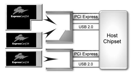
The ExpressCard architecture is modular and extensible, allowing for multiple slots as illustrated here.
